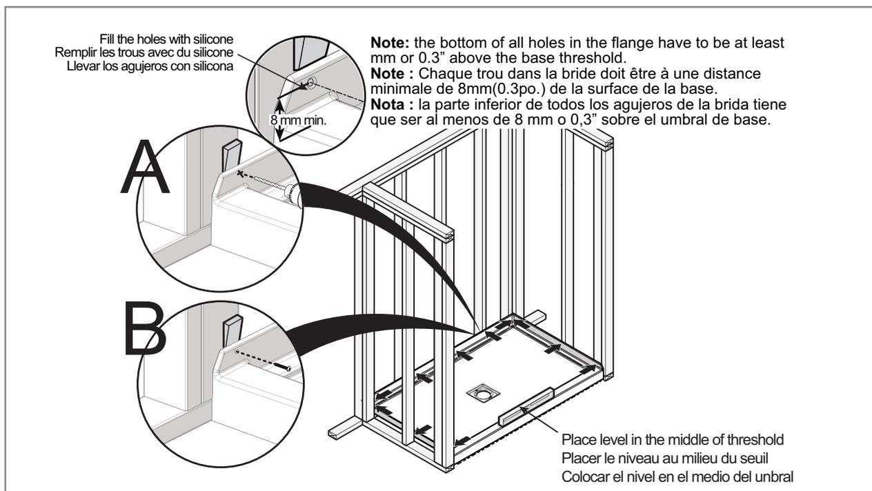
Seal the joint between the unit and the wall covering with a bead of silicone. Leave a 1" gap on the sides to work as a weep hole as shown.
