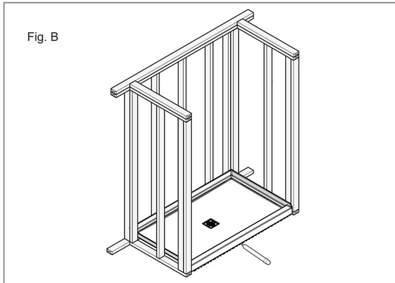
Making sure that the installation is level (position your level in the middle of the thresholds), reposition the base in place for the cement to take the form of the base perfectly while it is still wet. If you need to stabilize the unit while the cement is drying, use wooden shims.
